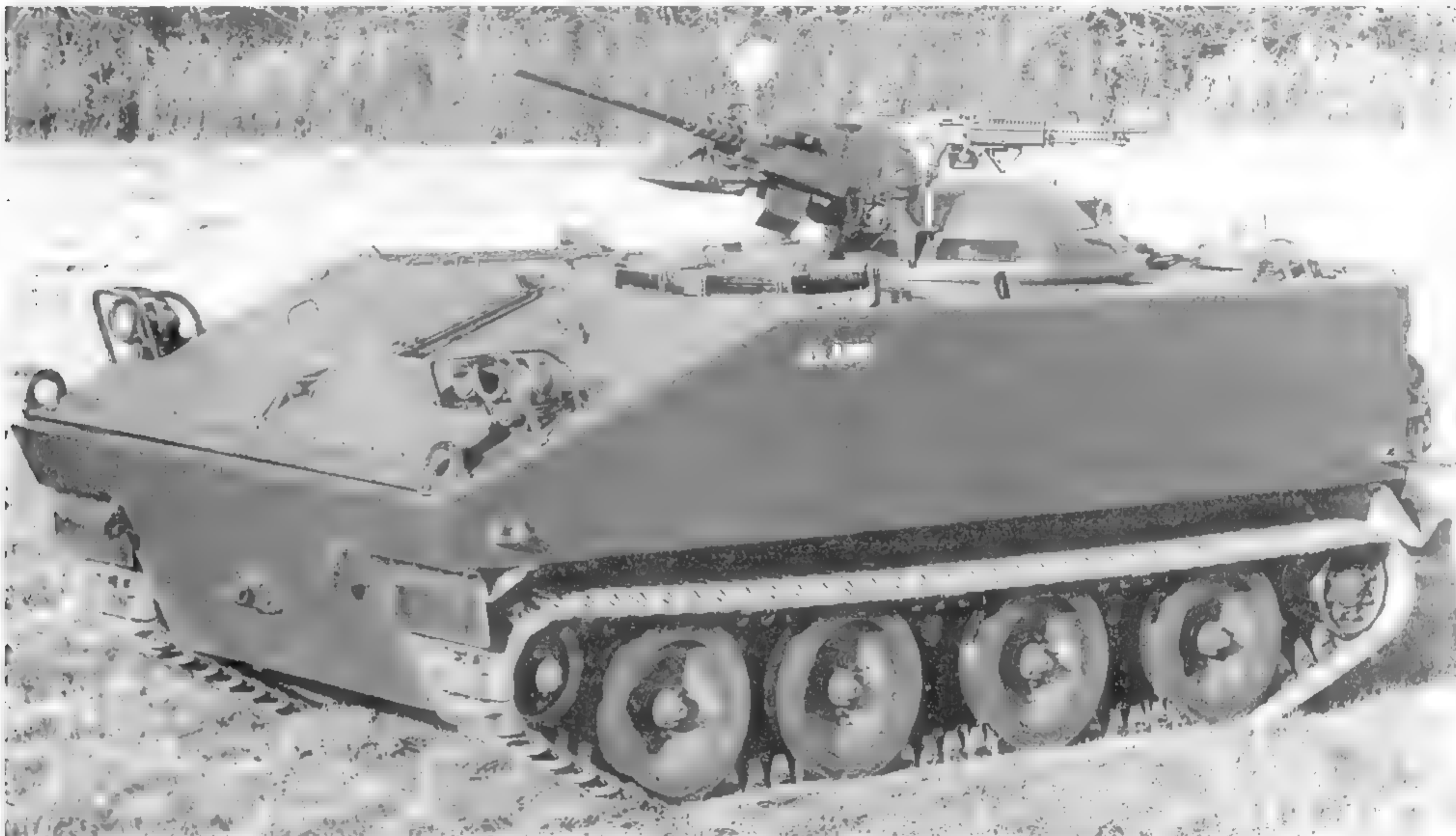
An M114A1 equipped with a turret mount for the commander's .50-caliber machine gun allowed him to fire the weapon from inside the vehicle. The original M114 machine gun installation required the commander to expose himself to hostile fire in order to operate the weapon. (U.S. Army photo)
